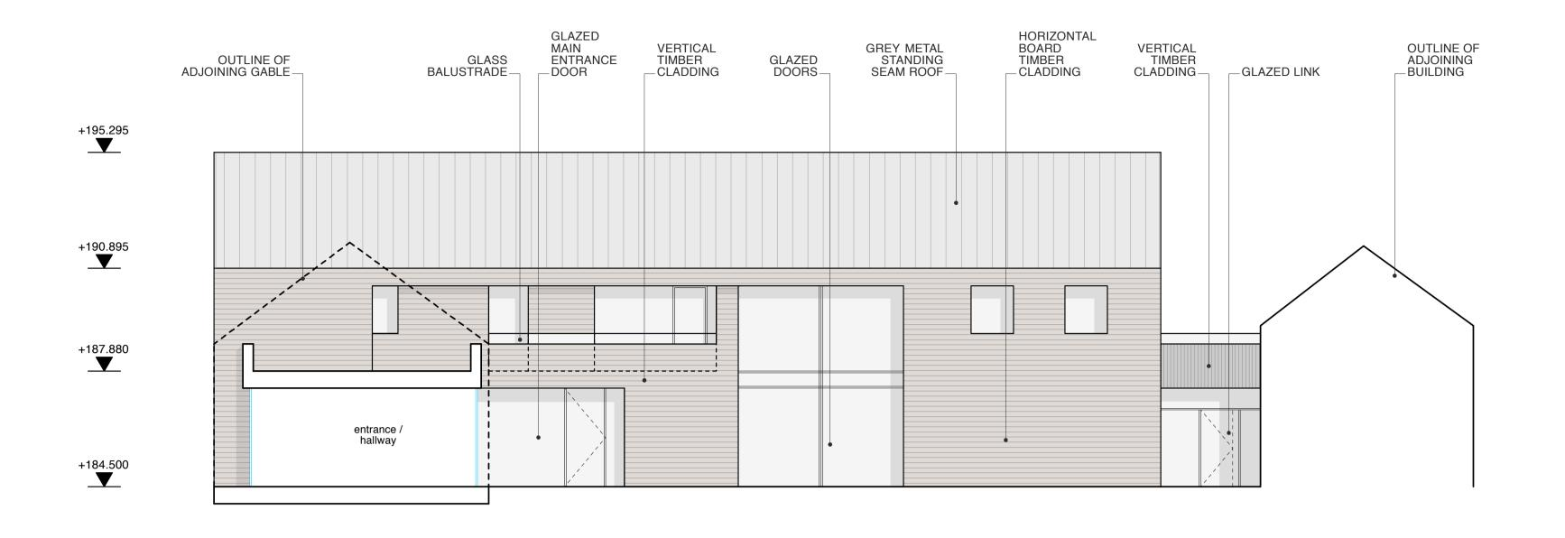
DATUM 180.00 **Elevation A** Proposed South Elevation
