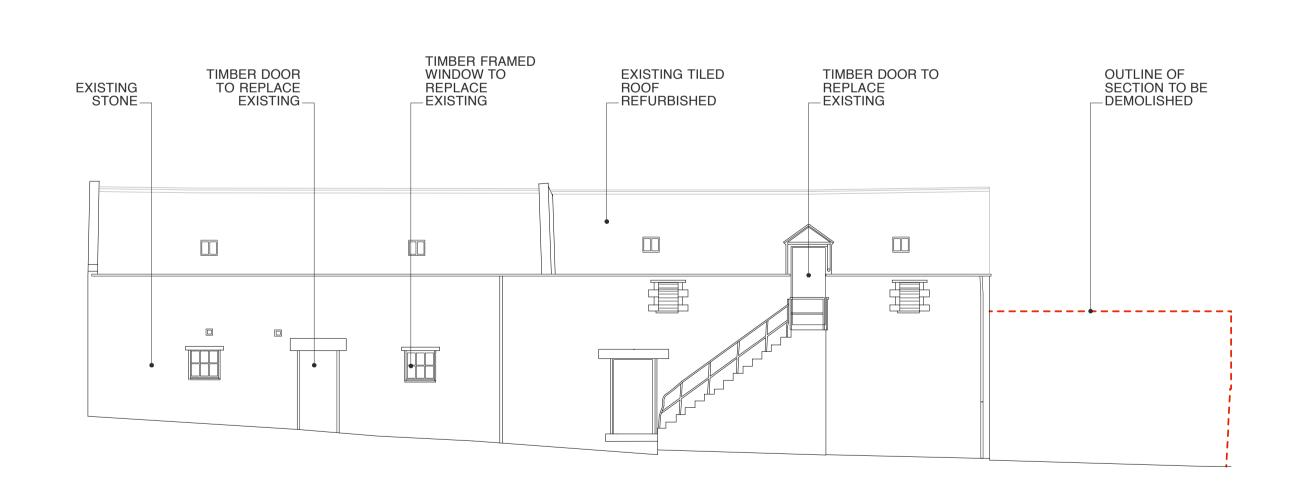
Elevation G Proposed South East Elevation DATUM 180.00
